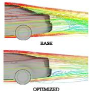
Fig. 13. Flow around the models
