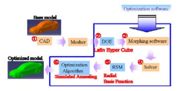
Fig. 1. Schematic of the optimization flow
